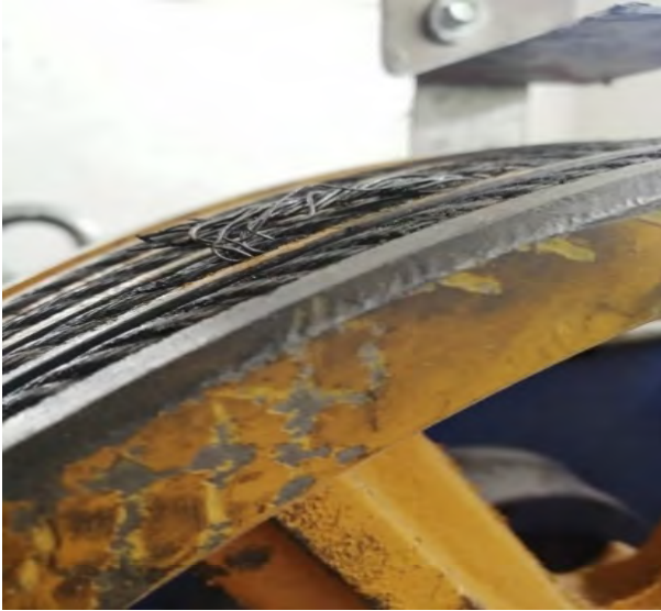
Picture 1. Deformed rope and worn pulley
