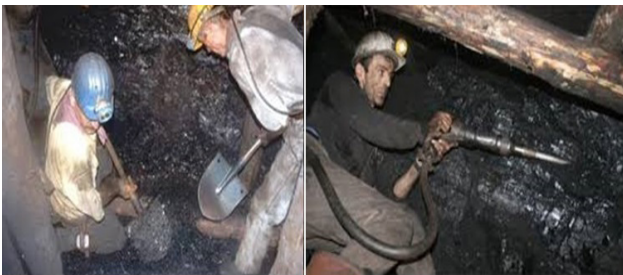
Figure 19. Manual excavation and loading work of miners in underground mines
