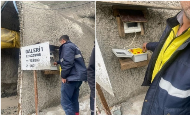
Figure 18. Safe detonation of blasting holes from outside the mine by a blasting specialist
