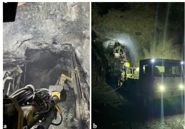
Figure 17. The situation of the drilling machine for boring holes[a], and the explosive filling of the blasting holes to produce the mine [b]
