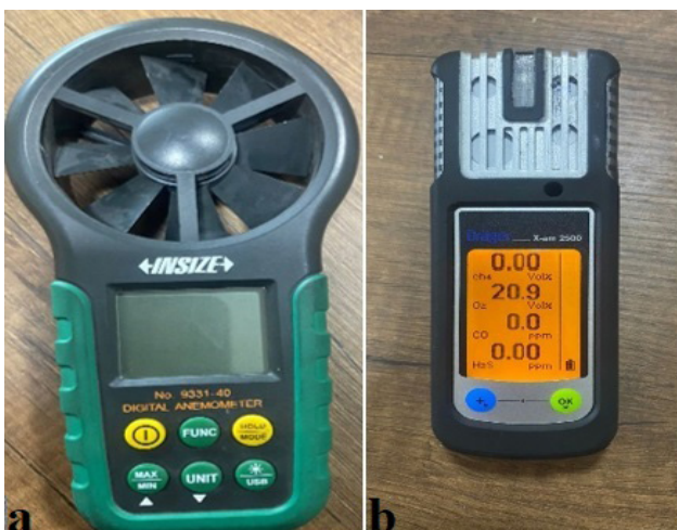
Figure 5. Manual air velocity measuring device [a] and gas measuring device [b]
