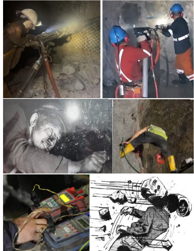
Figure 16. The process of miners manually opening blast holes, filling them with explosives and firing by blaster in underground mining
