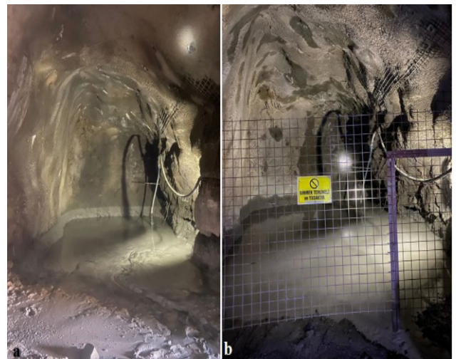
Figure 22. The pool where underground water accumulates (a) is covered with a wire mesh to prevent any dangerous situation (b)
